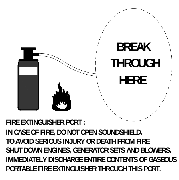
Fig. 2: Fire extinguisher port.
